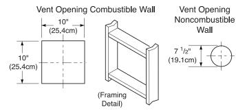
Figure 24 - Vent Opening Requirements
